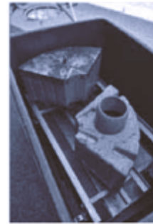
3. Put the other filter elements into the box
