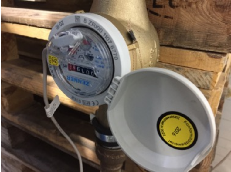
Figure 9. Flow-meter for low flow rates (sediment removal test)
