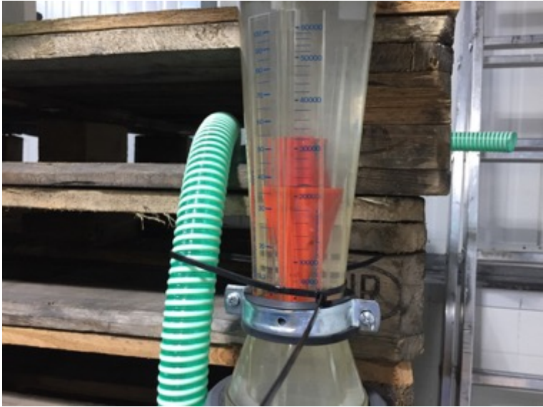
Figure 8. Flow-meter for high flow rates (scour test)
